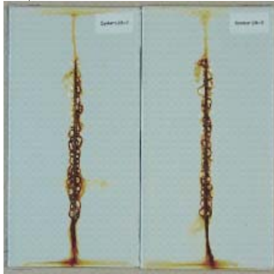
Photographs of SigmaFast 302 top coated with a highly durable finish. Tested to Norsok M501 standards. 4200 hours of salt spray, wet/dry cycle tests. Corrosion from the scribe is less than 2 mm.
